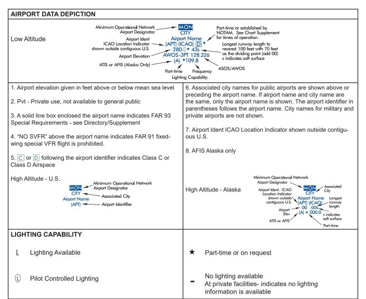
A symbol between the airport elevation and runway length means that runway lights are in operation sunset to sunrise. A symbol indicates there is Pilot Controlled Lighting. A symbol means the lighting is part-time or on request, the pilot should consult the Chart Supplement for light operating procedures. The Aeronautical Information Manual (AIM) thoroughly explains the types and uses of airport lighting aids.
