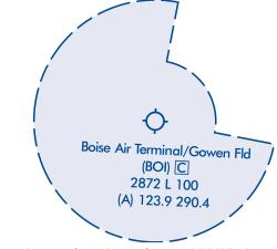
That airspace from the surface to 4,000' (unless otherwise designated) above the elevation of selected airports (charted in MSL). The normal radius of the outer limits of Class C airspace is 10NM. Class C airspace is also indicated by the letter C in a box following the airport name.
