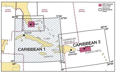
The chart symbols used on the Caribbean Charts are similar to those used in the Sectional and Terminal Area Charts, the major difference being in scale. The Caribbean VFR Chart scale is 1:1,000,000 versus the Sectional Chart Scale of 1:500,000 and Terminal Area Chart Scale of 1:250,000. Chart symbology will appear smaller on the Caribbean VFR Charts.
